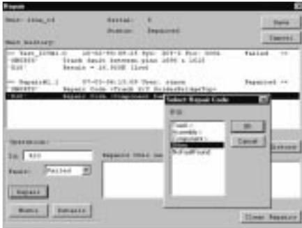
This is an interactive environment where operators enter a unit identifier to view and analyze full unit histories on screen. Fault and optional device information (stock codes, nominal values) is displayed. Users may be grouped (for example) as Repairer or Inspector, and allocated Repair Codes or Fault Categories. These codes, used to classify test failures, are entered from bar-code or on-screen lists. Comments can be added per repair session, or (depending on user configuration) per repair.
